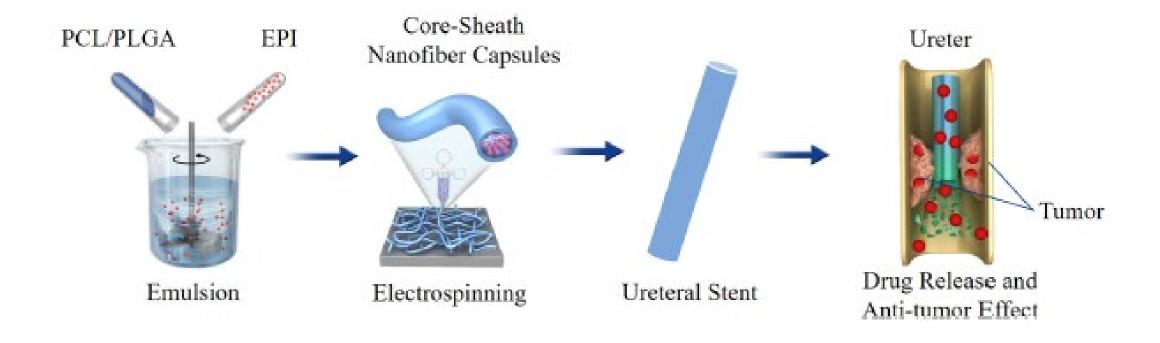
Schematic illustration of preparation and antitumor effect of Epirubicin-loaded BUS
